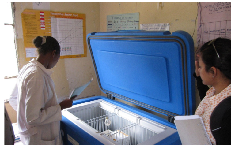
CCE: TCW 3000AC, capacity 150 liters, often used at larger health facilities
