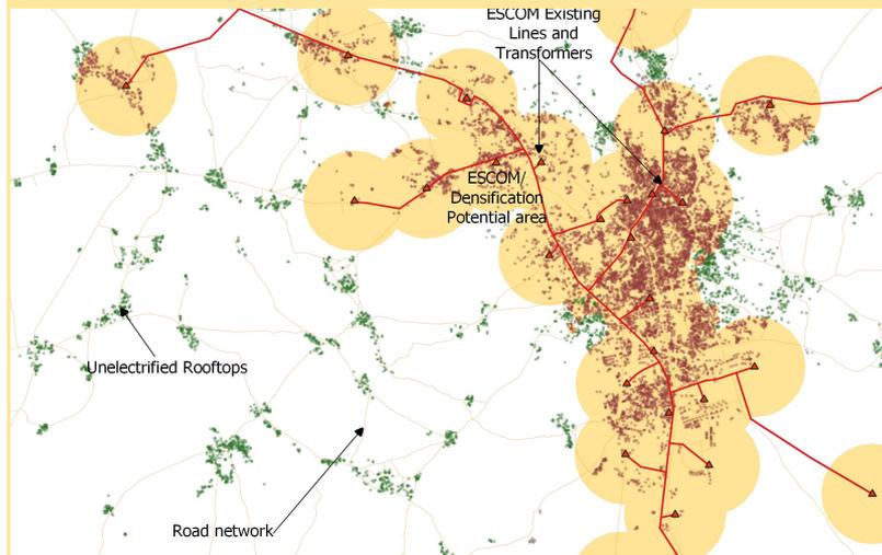
**Clustering Algorithm:** unelectrified structures beyond the densification boundaries are grouped into clusters for evaluation of grid expansion or off-grid electrification.
