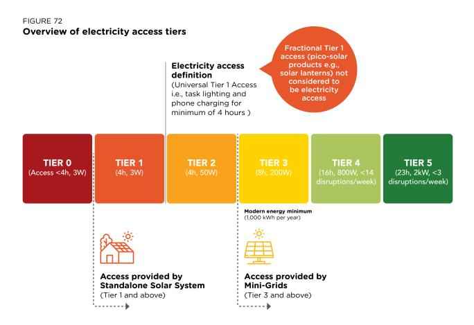
**Mapping technologies to tiers:** While all three technologies mentioned above enable at least Tier 1 access, grids and mini-grids are mapped to higher tiers than SHSs. In most cases, access to the grid maps to Tier 4/5 access based on the MTF, access to mini-grids maps to Tier 3/4 and access to SHSs map to Tier 1/2. Note that pico-solar products such as solar lanterns map to partial Tier 1 access. However, contrary to the 2019 Taking the Pulse
