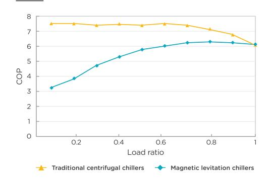
Source: Manufacturer's test results (Cooling water inlet 30°C, chilled water outlet 7°C)
