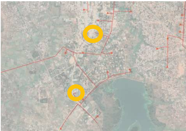
Figure 1: MV lines without transformers
