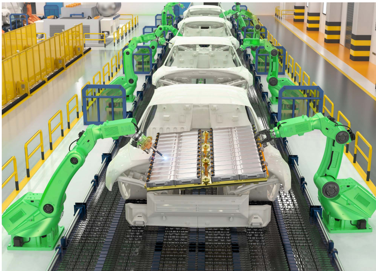
FIGURE 6: Automated car factory with 3D-rendered robot assembly line and electric car battery module on platform. 18
